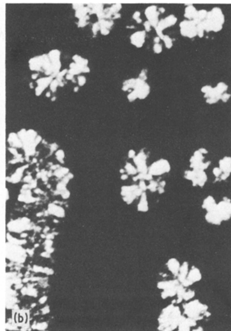
Figure 4 Micrographs of \text{Li}_2\text{O}\cdot 2\text{SiO}_2 spherulites formed in massive samples heat treated at (a) 564^\circ\text{C} for 120 min, (b) 564^\circ\text{C} for 420 min (c) 650^\circ\text{C} for 90 min. Crossed nicols: (a) \times 160 , (b) \times 25 and (c) \times 63 .
