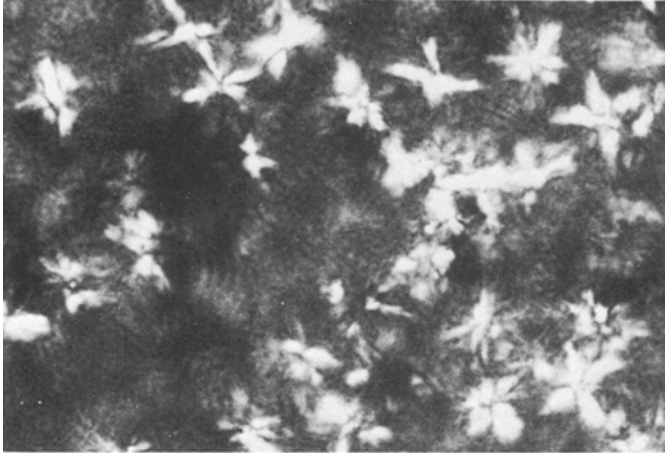
Figure 5 \text{Li}_2\text{O} \cdot 2\text{SiO}_2 spherulites formed in a thin film sample heat treated at 650^\circ\text{C} 5 min. Crossed nicols, \times 160 .
